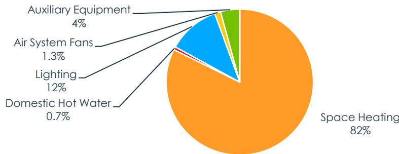
From the figure above, space heating is the end use that consumes the most energy at the facility with 81%. This is to be expected as there is fuel and electric sourced heating equipment on site and represent the largest opportunities for energy savings. Lighting is the next largest end user with 12%. Auxiliary equipment, air system fans and DHW make up the remainder with a combined portion of 6%.
