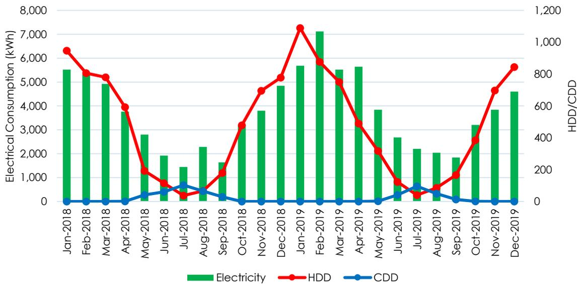
The figure shows that electricity consumption peaks in the winter months which is to be expected as there is multiple sources of electric heat and the facility is located in a heating dominated climate. There is a baseload of roughly 2,000 kWh/mo which can be attributed to DHW heating, lighting, plug loads, and exhaust fans.
