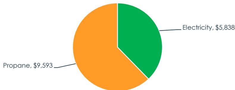
Electricity has been estimated to account for approximately 28% of all energy consumed at a cost of \$5,838 while propane accounts for the other 72% at a cost of \$9,593. The cost per energy metric for propane and electricity are \$23.37/GJ and \$37.36/GJ respectively.
