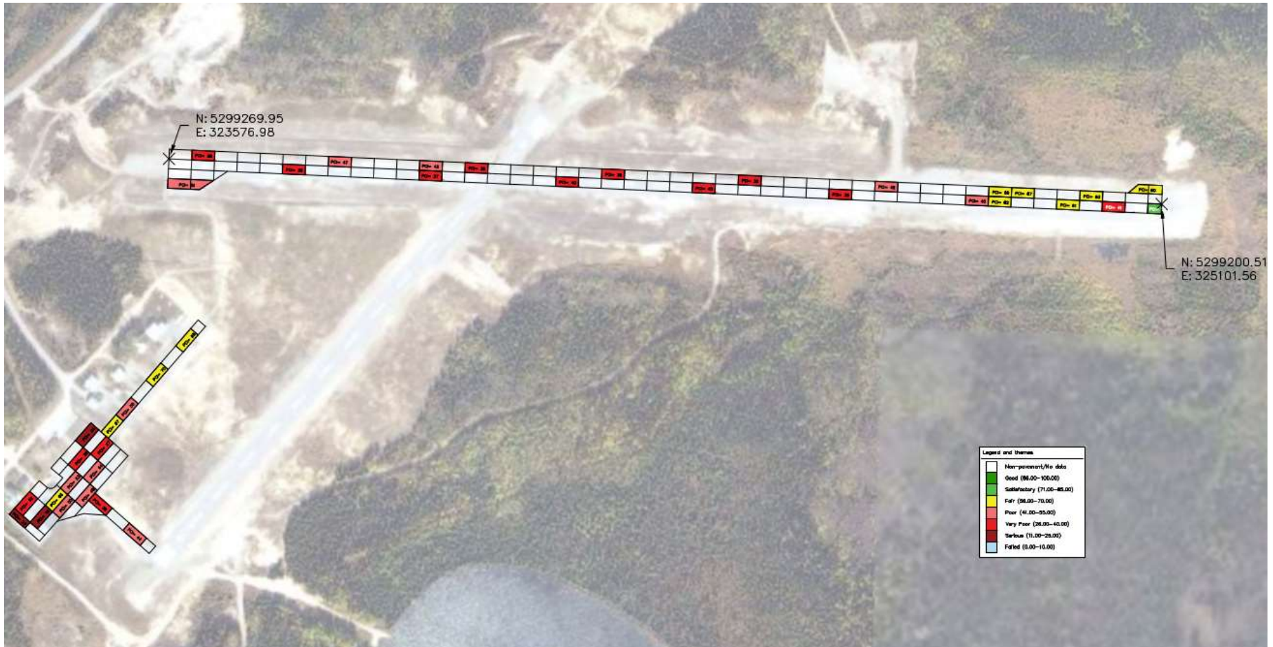
Figure 3-19 The PCI results for Each Sample Unit
