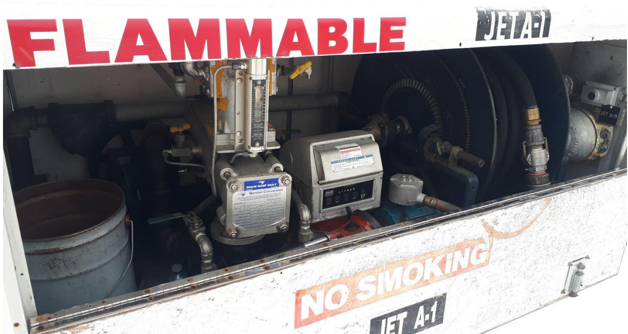
Jet Fuel Dispenser and Meter
